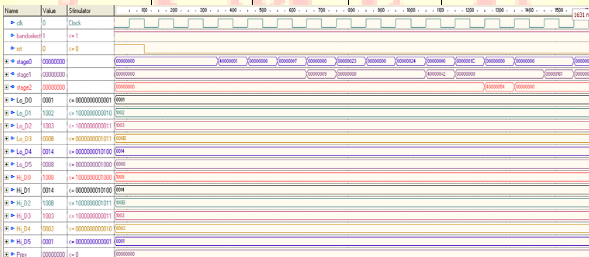
Figure 12: Simulation waveform for Daubechies3 when band select '1'-
